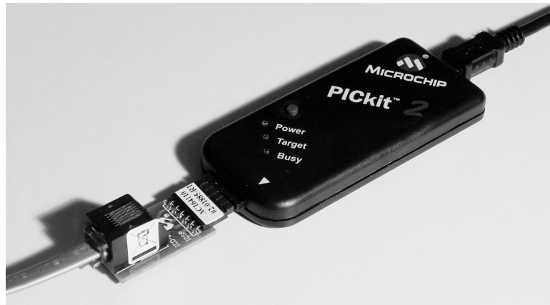
PICKit 2 shown with AC164110 RJ-11 to ICSP adapter including cable (attached)
